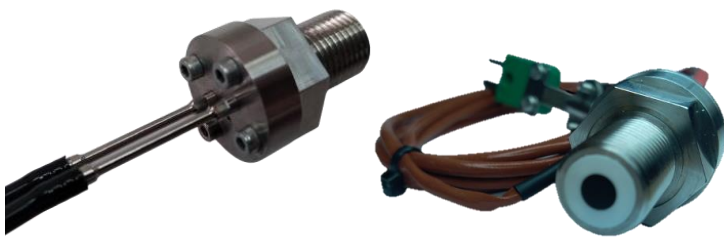
Figure 1 CHF heat flux sensors are very compact despite their cooling structure. They are able to work in continuous mode at high flux levels ( >MW/m^2 ), without any degradation.
